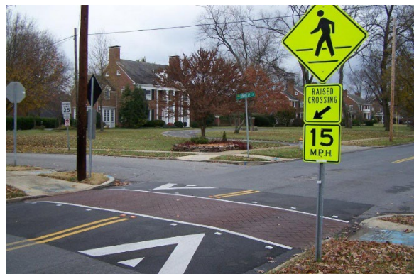
Figure 9: Raised Crosswalk (Source: Google)
