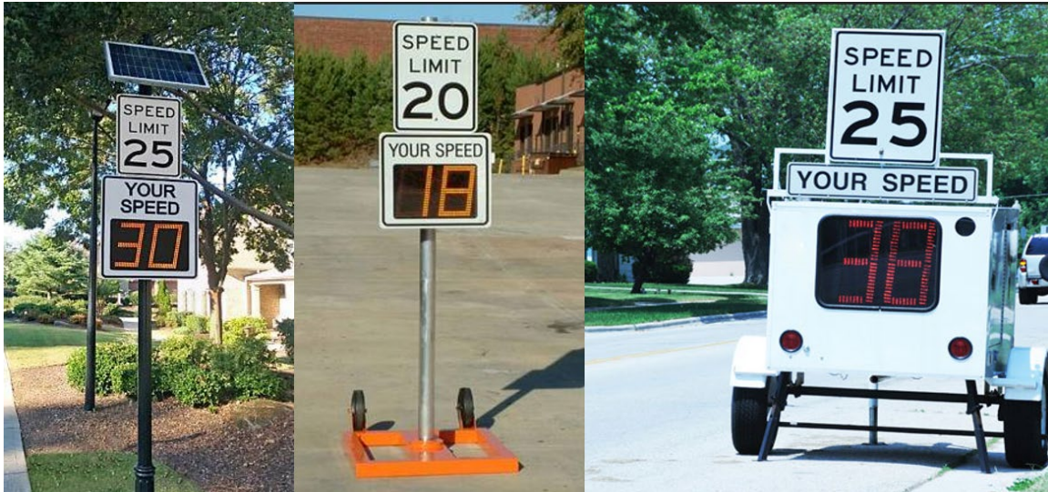
Figure 6: Speed Feedback Signs (Left – Permanent Fixture; Center and Right – Temporary Installments)
