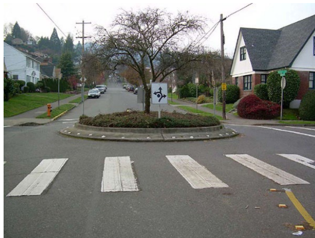
Figure 7: Neighborhood Traffic Circle (Source: FHWA Traffic Calming ePrimer)
